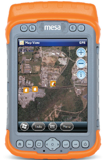
Mesa Geo 3G running ArcGIS Mobile software to map GPS coordinates of structures damaged by the Tuscaloosa tornado.
