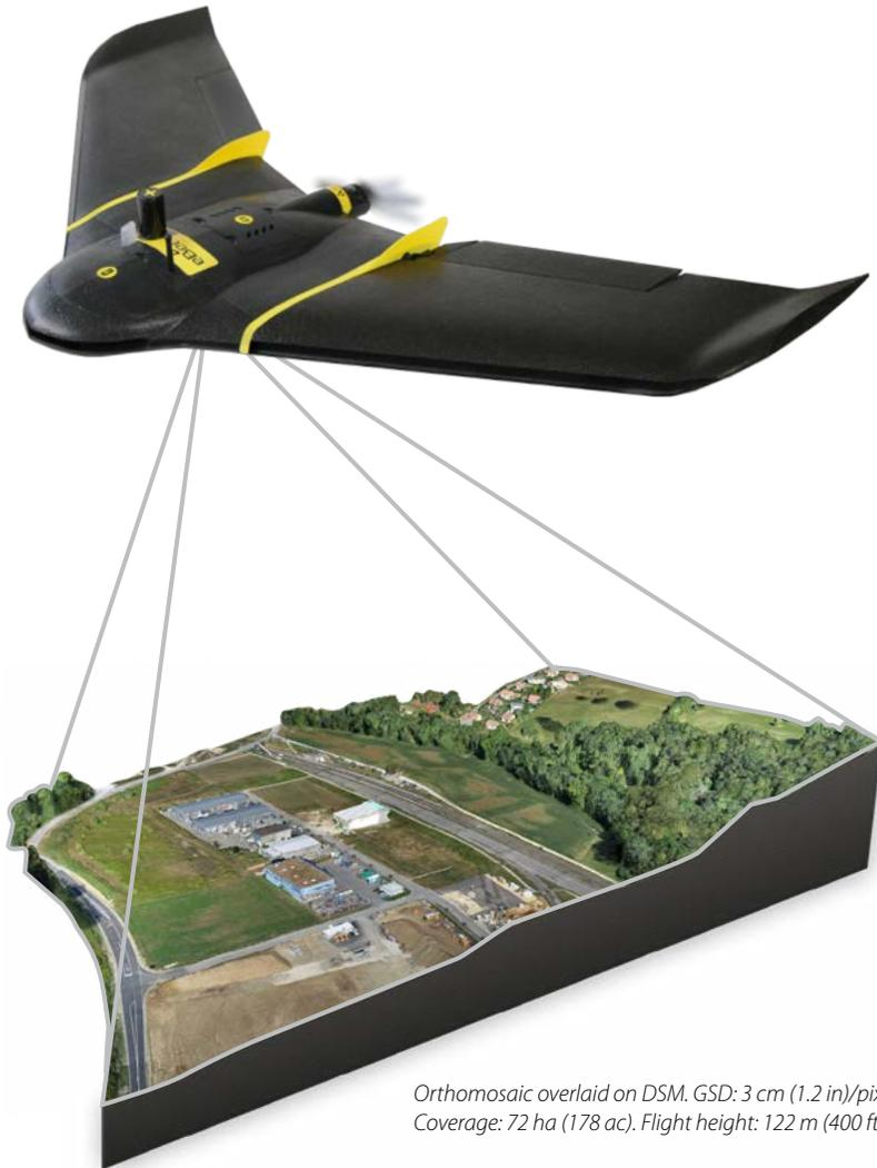
Orthomosaic overlaid on DSM. GSD: 3 cm (1.2 in)/pixel.
